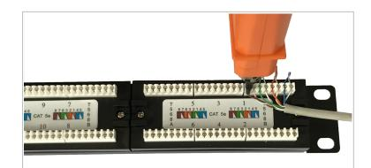
Use an impact tool to punch in the wires and connect them into the IDC connectoron the back of the panel
