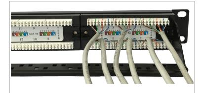
Lock the support bar onto the rear of the panel
